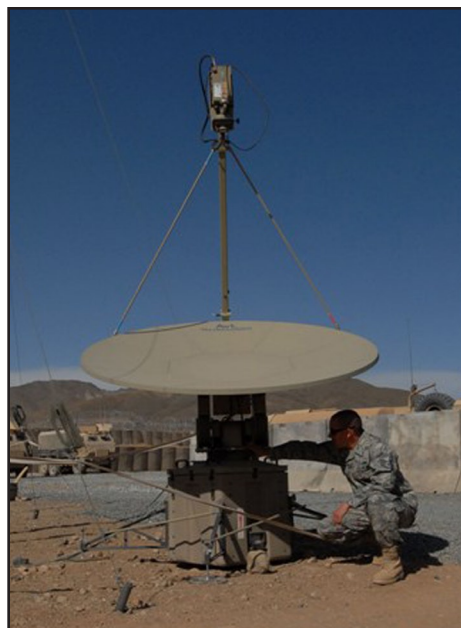
Air Force Staff Sgt. Jeremy Emond inspects the satellite dish of the Virtual Secure Internet Protocol Router, Non-secure Internet Protocol Router Access Point system at during his routine inspection at Combat Outpost McClain.
