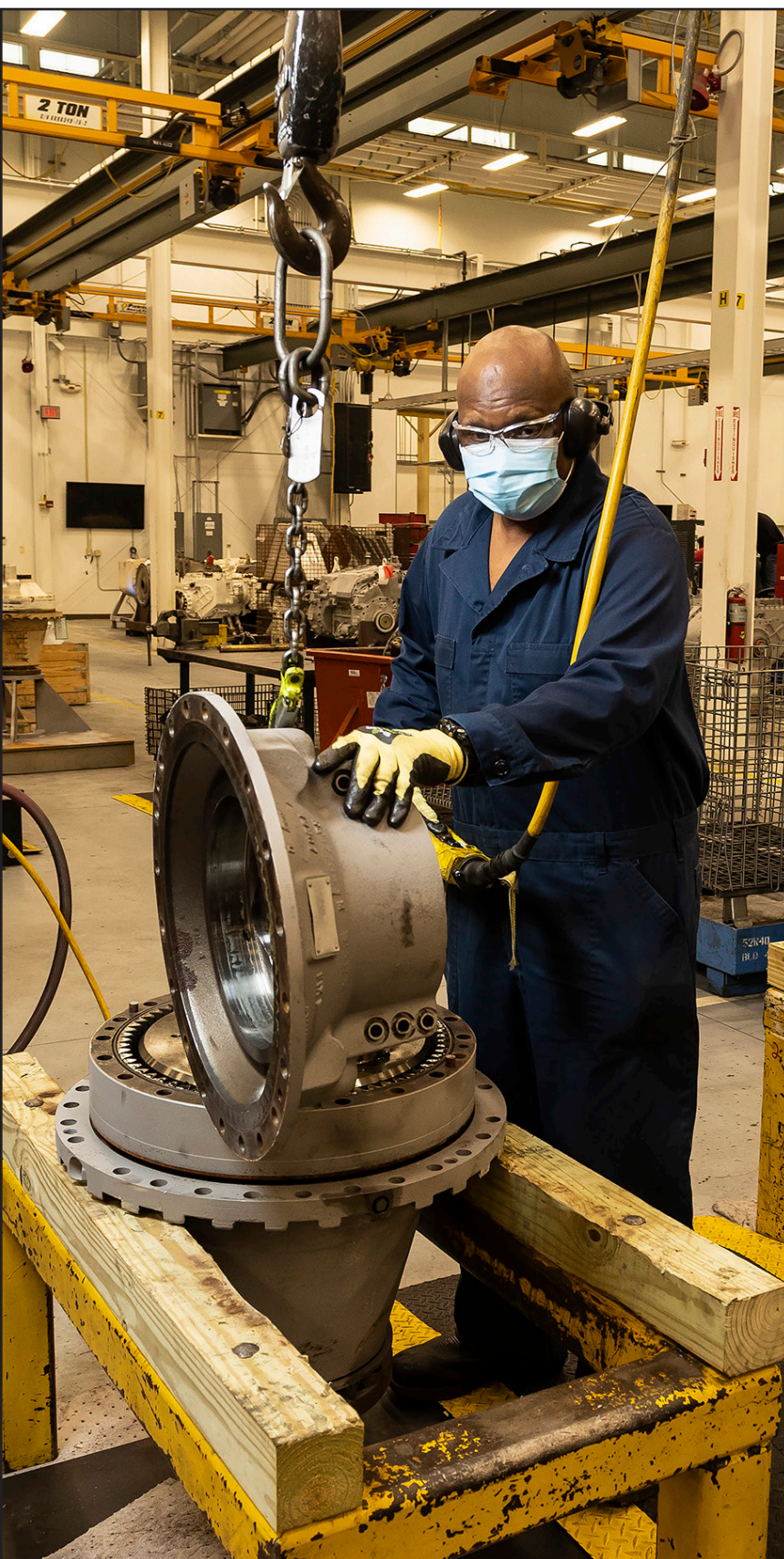
Nathaniel Williams, a heavy mobile equipment mechanic, disassembles a final drive for the M1 Abrams in the Final Drive Branch at Anniston Army Depot.
