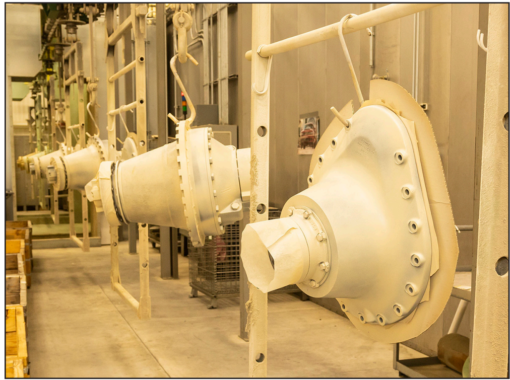
A row of final drives for the M1 Abrams hang on a paint conveyor where they await a final coat of paint.
