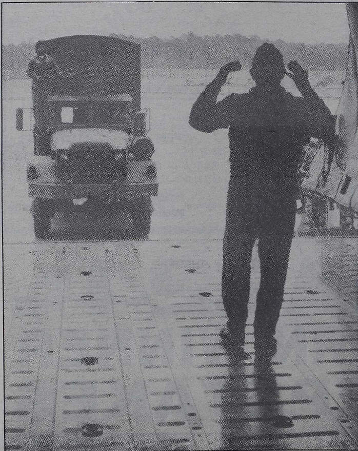
An Air Force loadmaster directs a Headquarters Battalion's 2d Marine Division Marine in driving his vehicle aboard a C-5A. (Photo by SSgt. Marie Johnson)
