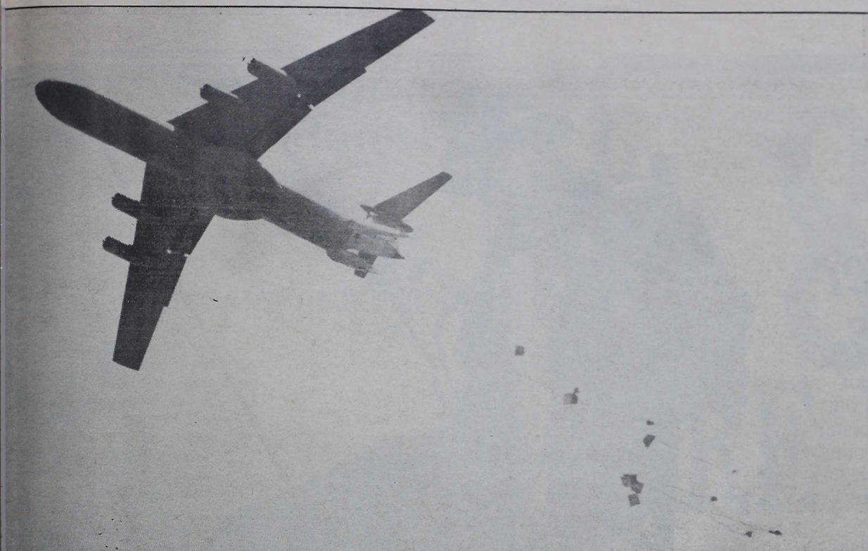
(Left) An Air Force C-141 drops six cargo delivery loads weighing about 1,500 pounds each during a joint exercise recently. (Below right) The cargo bundles float down, using G-12 cargo parachutes. The CDS bundles landed together in Drop Zone Falcon, making the drop a success. (Photos by PFC K. J. Bloomer)
