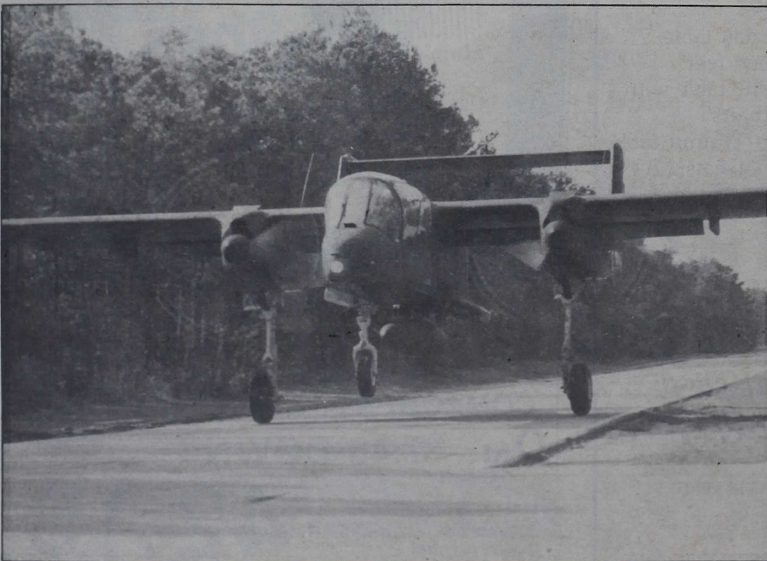
In the Short Take-Off and Landing configuration, an OV-10 Bronco from Marine Observation Squadron, home-based at Marine Corps Air Station, New River, performs road operations at Lyman Road. (Photo by Sgt. N. H. North)
