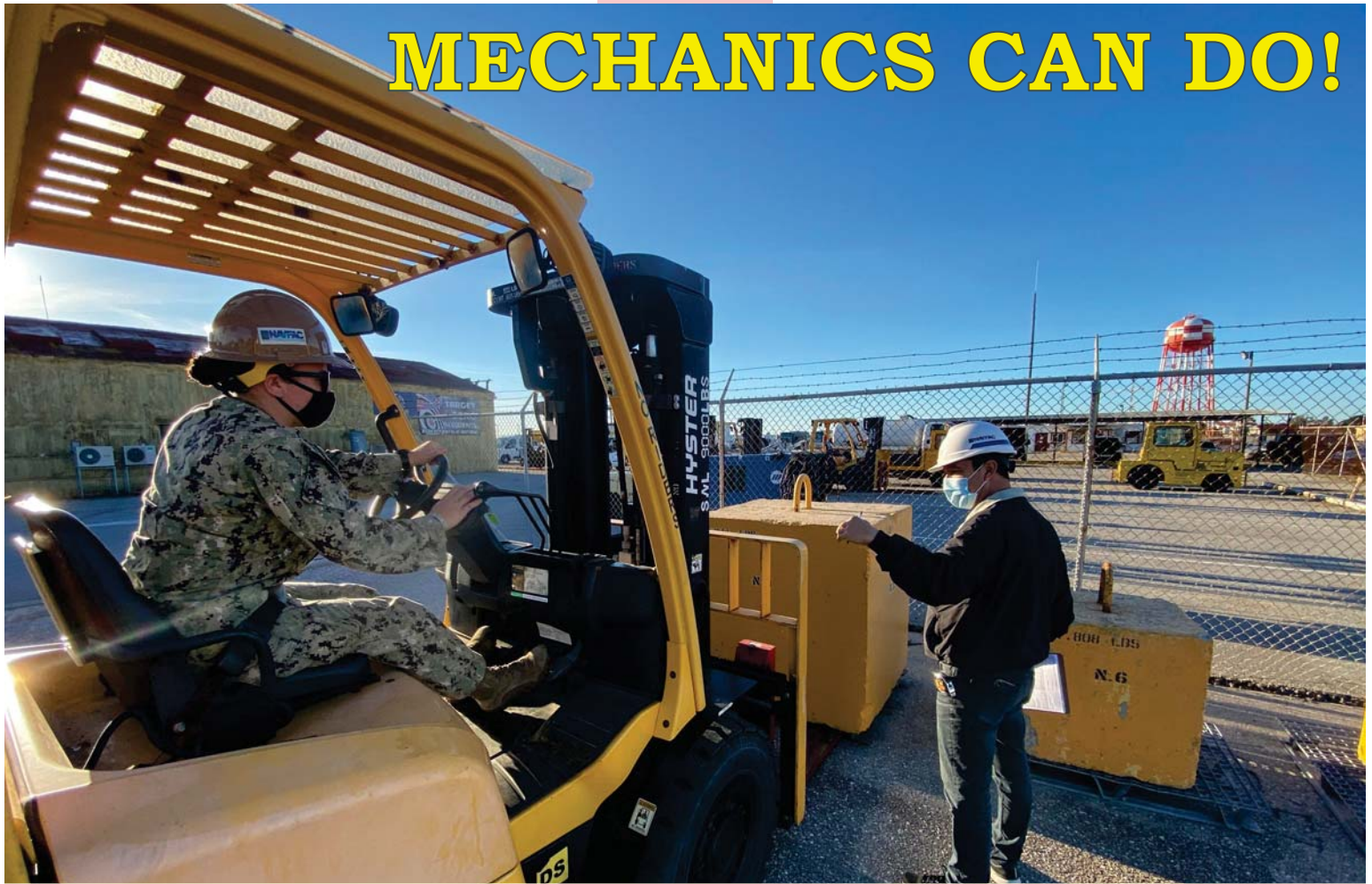
Above and Below: CM3(SCW/EXW) Teagan Lapping (left), conducts a forklift inspection and certification along with Alberto Vazquez (right) at the testing area within the motor pool area of PWD Rota, Spain on March 12th, 2021.
