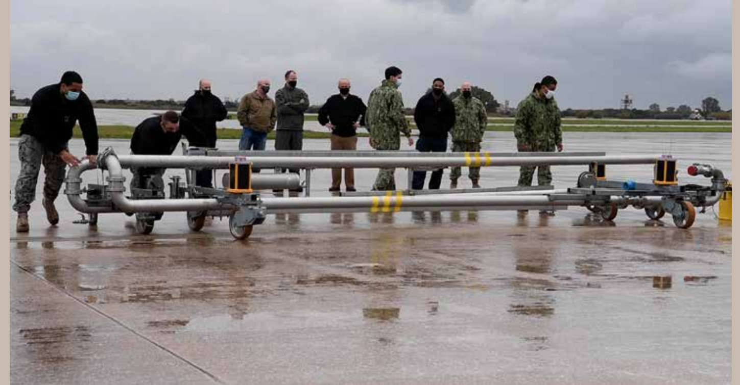
Above: Aviation Boatswain's Mate (Fuels) 2nd Class (ABF2) Dashaun Lewis (left) and ABF3 Christopher McConnell (second from left), retract a refueling pantograph to demonstrate how to position the equipment for proper refueling operations at Naval Station (NAVSTA) Rota, Spain. Lewis and McConnell are assigned to NAVSUP FLC Sigonella. —photo by John Owen
