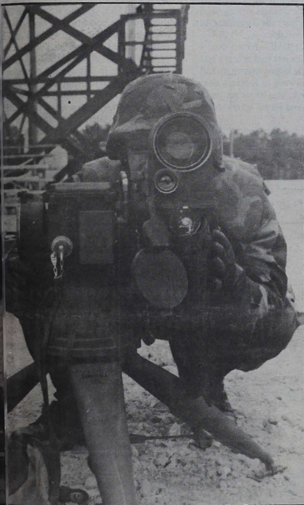
Stephen P. Ames, a radio operator with 3/6, sights in on a target with MULE. The laser operated MULE can pinpoint targets 2,500 meters away.
