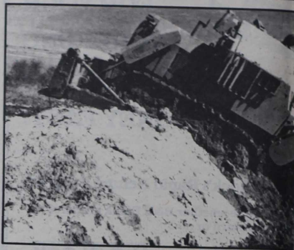
An armored bulldozer moves earth to make an anti-tank ditch passable for vehicles.
