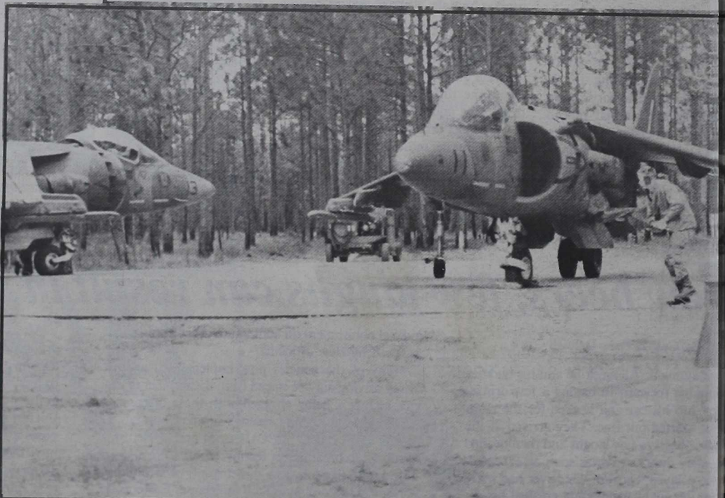
HARRIER HIVE— Crewmen from MWSS-272 from MCAS New River rush forward to refuel a pair of waiting AV-8B Harriers of VMA-231 from MCAS Cherry Point at a "Harrier Hive" on Lyman Road recently. The "hive" refueling procedure demonstrates the vertical-lift aircraft the capability of operating as close to the forward edge of the battle area as possible.
