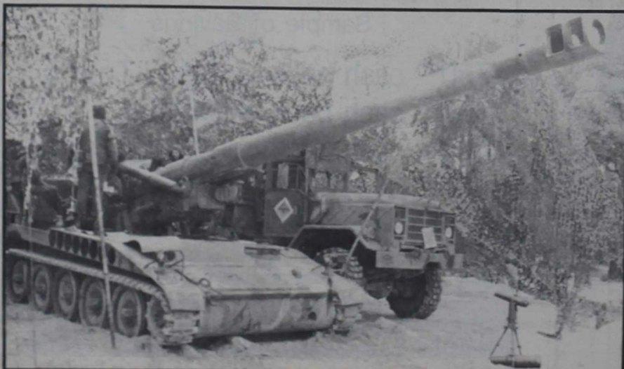
GOLIATH'S GUN —The M110-A1, 8-inch howitzer is the Marine Corps' largest gun. It shoots a round a distance of about 30,000 meters.
