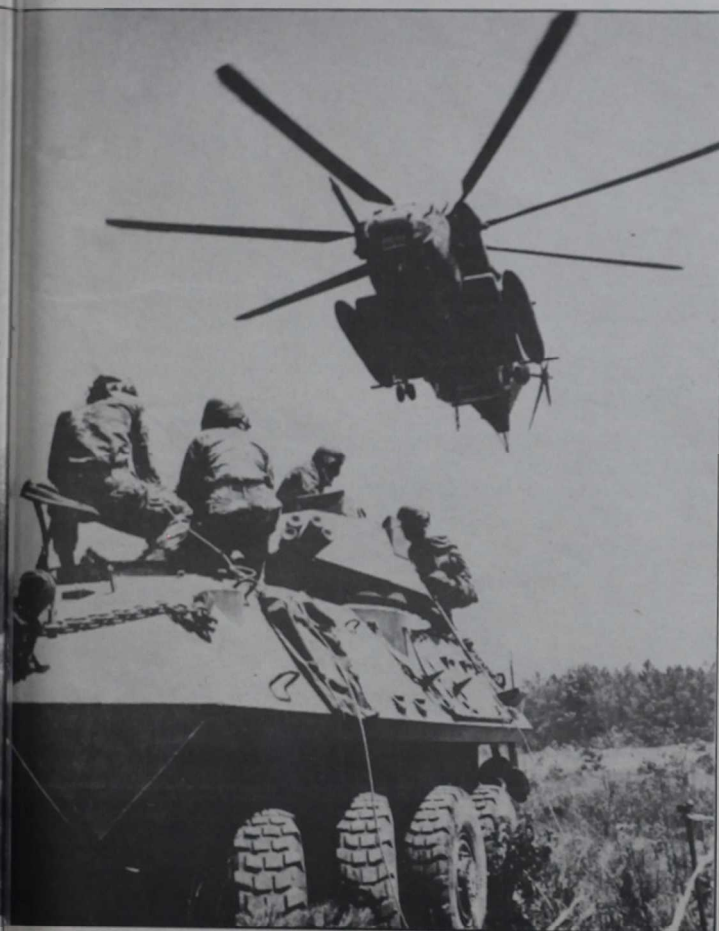
2nd LSB, gets ready to hook up an LAV for an external lift.
