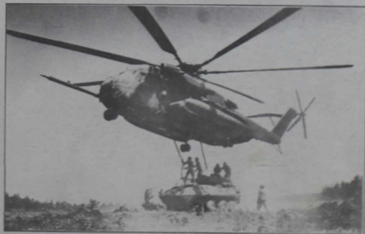
A Super Stallion hovers over an LAV during an external lift exercise.
