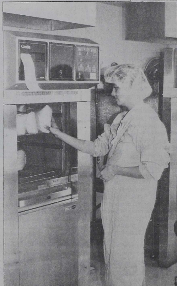
Petty Officer 3rd Class Catherine T. Bellamy places packaged surgical gowns into the autoclave for sterilization.
