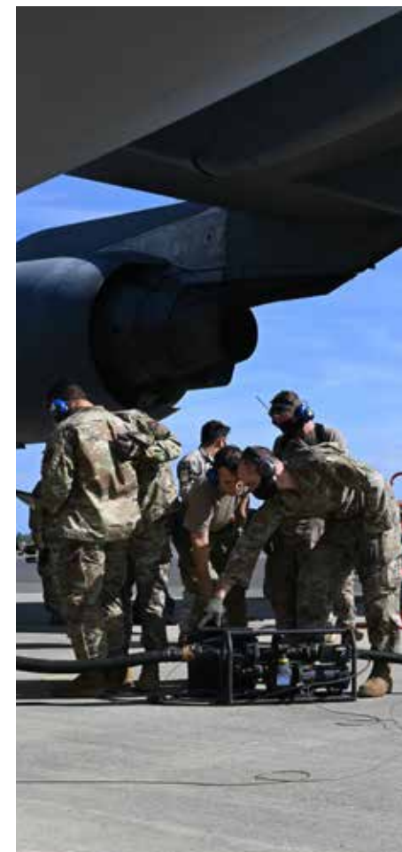
Airmen transfer fuel from a C-17 Globemaster III to an F-22 Raptor Feb. 25.
