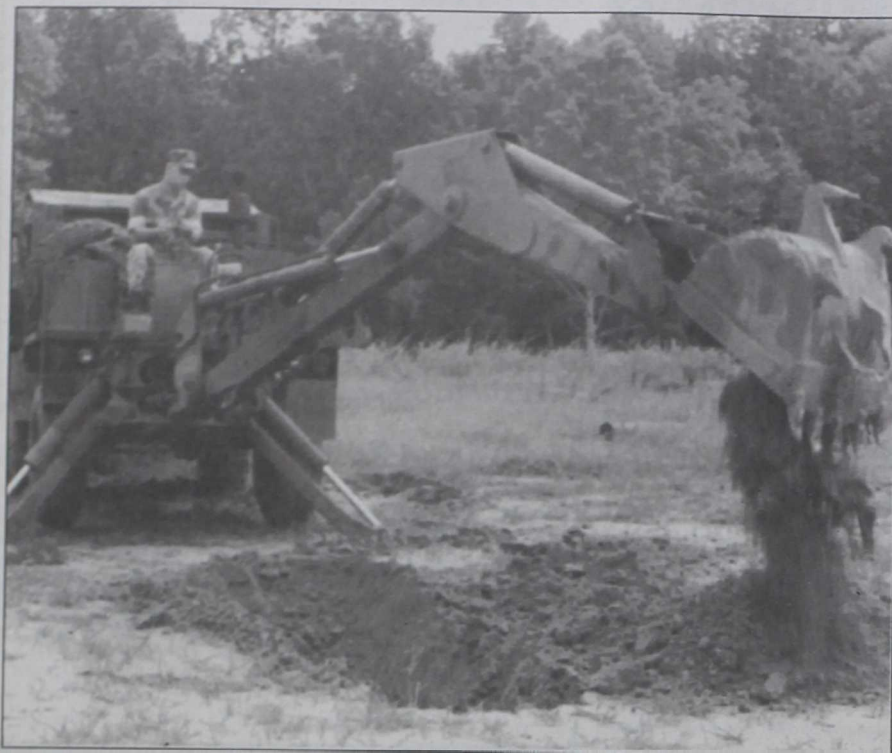
LCpl. Jeramiah Westerfield, 4th squad, Engineer Plt., uses a Small Emplacement Excavator (SEE) Tractor to dig a two-man fighting hole. The combat engineers honed their knowledge of constructing fortified positions during training at Fort A.P. Hill recently.
