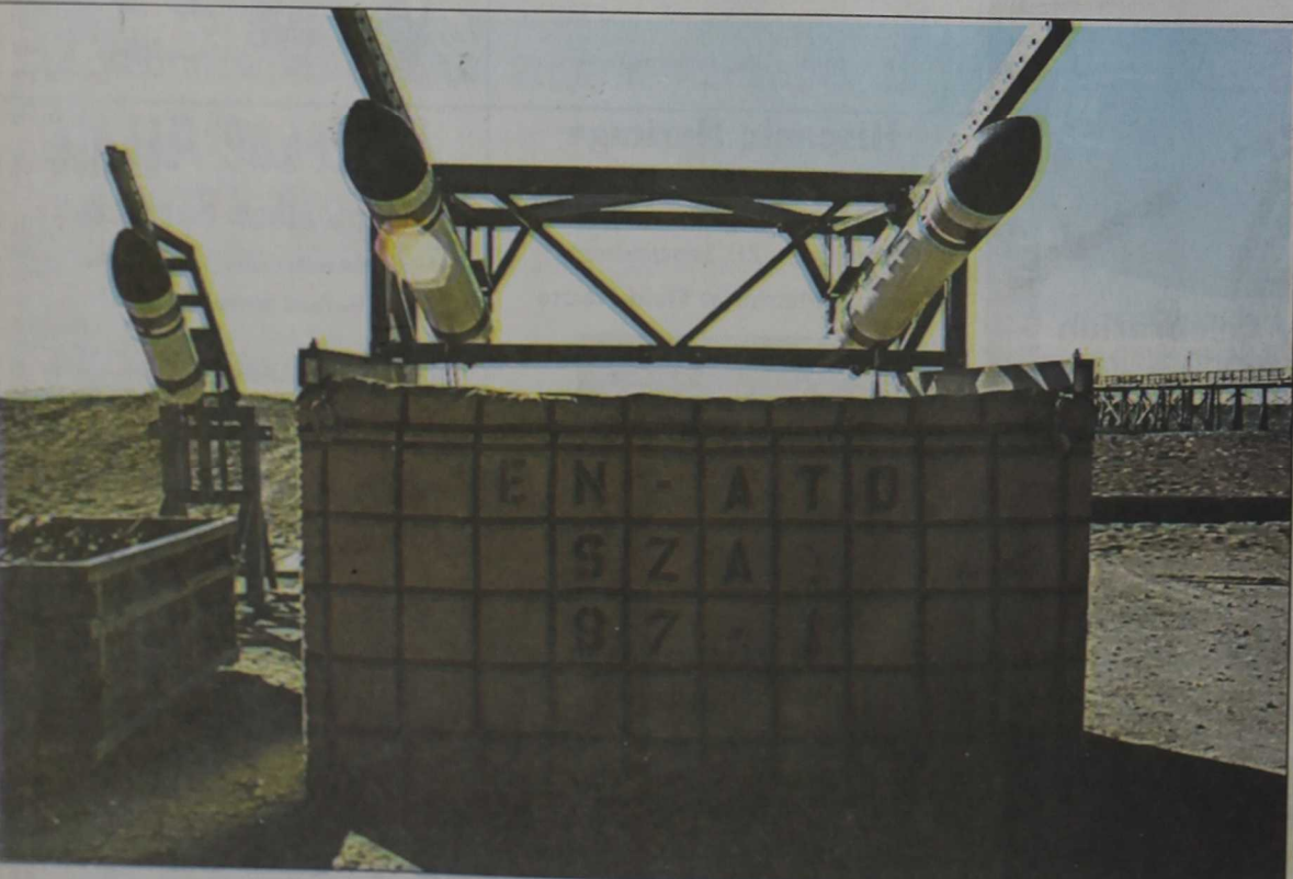
The explosive neutralization system is a line charge designed to be deployed from an LCAC.
