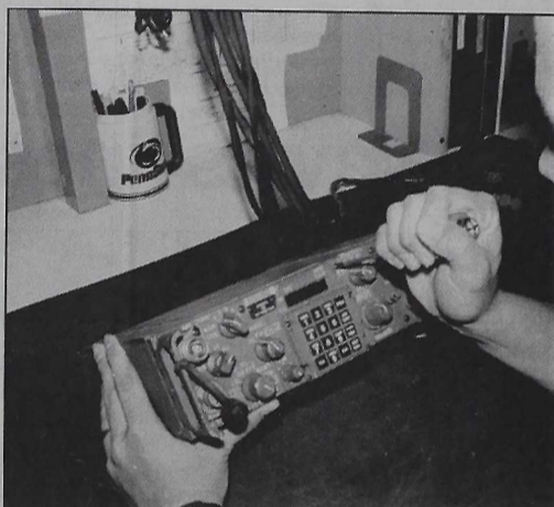
Cpl. Ozzie Agramonte, repairs a RT1523C SINGARS Radio.
