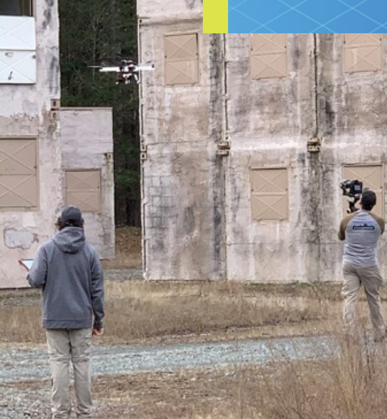
A small UAV with mounted chemical sensors was operated to conduct remote recon to detect chemical vapors. (U.S. Air Force photo by Pierce Jennings)
