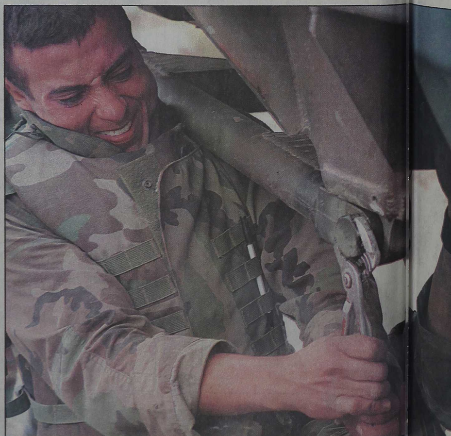
LCpl Jorge DeLaRosa and PFC Steven Drexler of Charlie Battery, 1st Battalion, 10th Marines. The artillery mechanics said the travel lock on the howitzer was stuck, and unless the bolt was to be lifted by the U.S. Army Chinook. It took the pair about 15-minutes and some axle grease to get the bolt to move.
