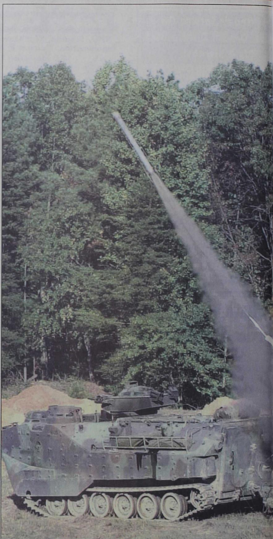
Marines from 2d Combat Engineer Bn and 8th Engineer Support Bn, fire an inert line charge.
