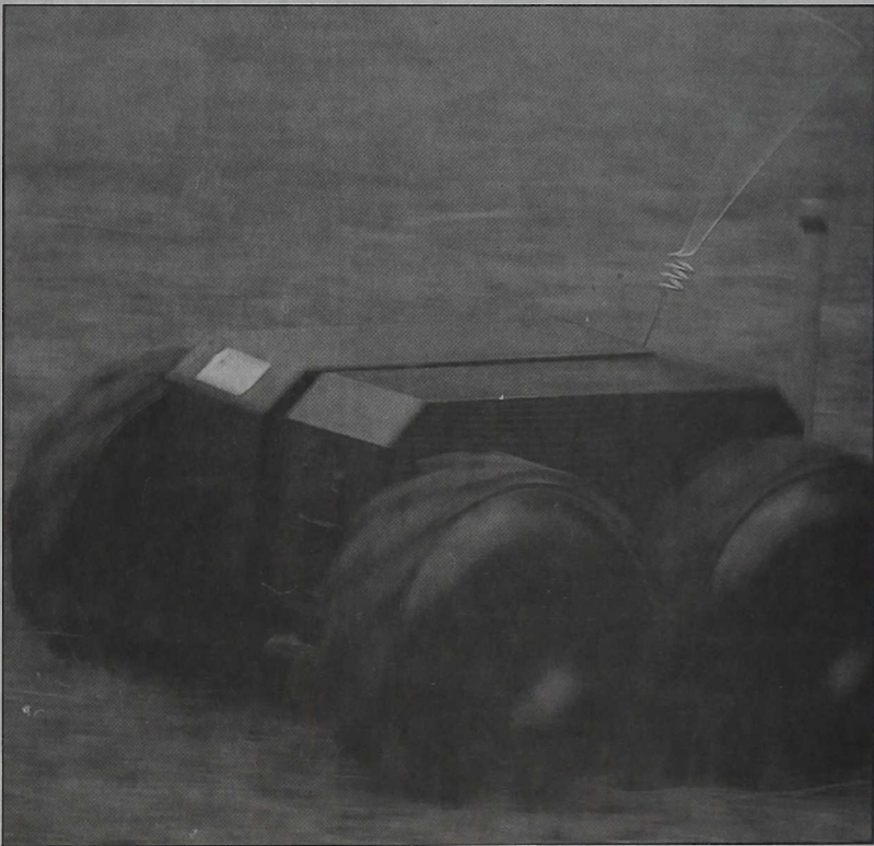
The rattler is one of the four robotic sensors that were used during Millennium Dragon exercise at Camp Shelby, Miss through Sept 13. It is 20 inches long, 22 inches wide and stands 12 inches tall. Its built in camera makes it teleoperated robot sending a live image back to the operator.
