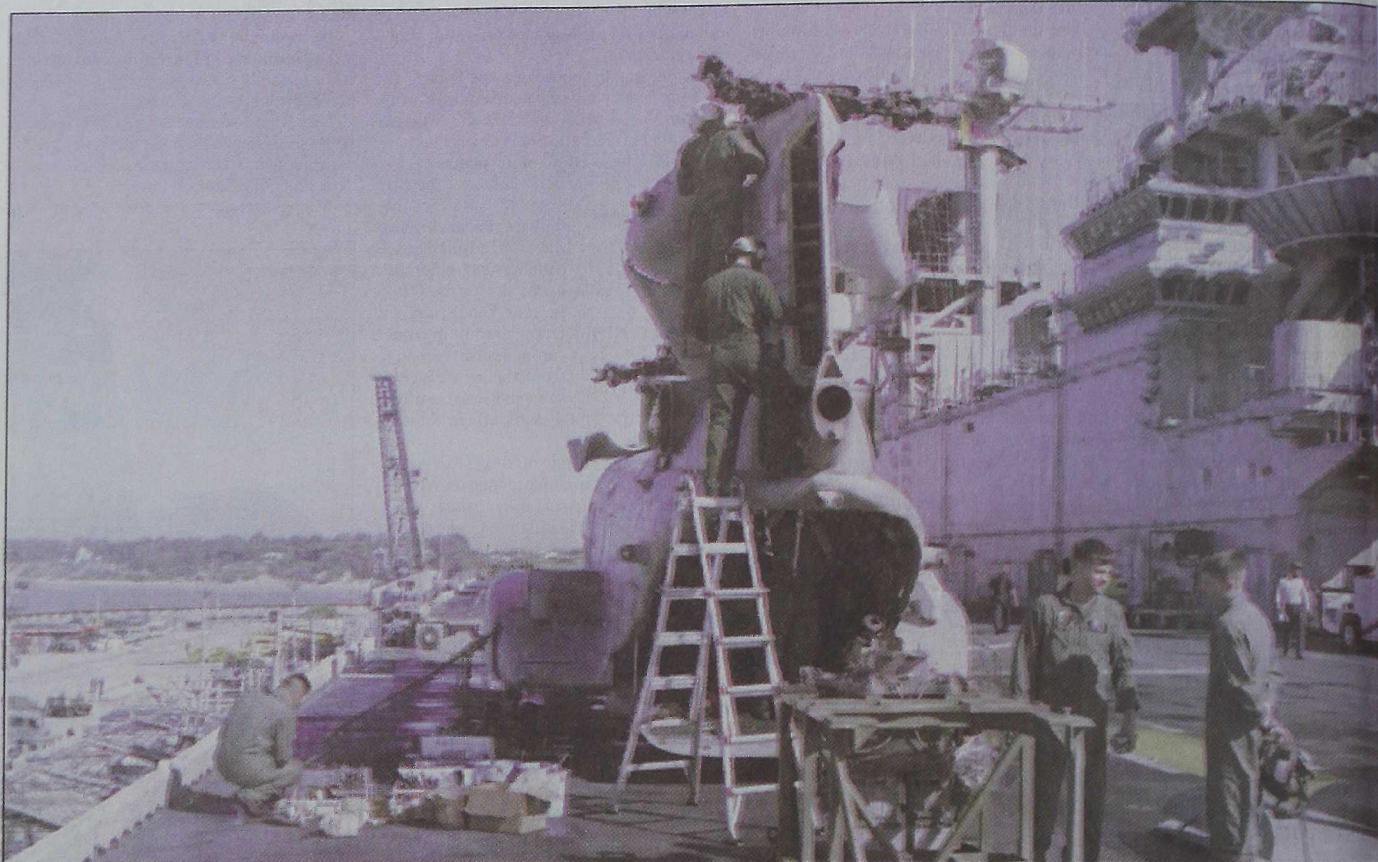
LCpl Robert Mabry , left, 46 mechanic, HMM-263, from Pocahontas, Va., and Cpl Robert Gallipeau , 46 mechanic, from Syracuse, N.Y., inspect and perform maintenance on the rear rotor assembly of a CH-46E helicopter.
