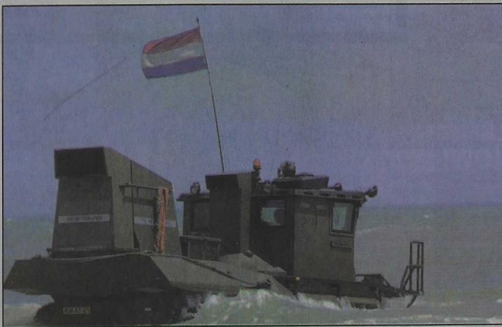
The SAMSON recovery vehicle of the Dutch Royal Marines can go into 7 ft of surf to recover or push out landing craft. The first such recovery vehicle is called Hurcules. Both are armored plated. Windows are 2in of bullet proof glass. Two more will be added to inventory next year.
