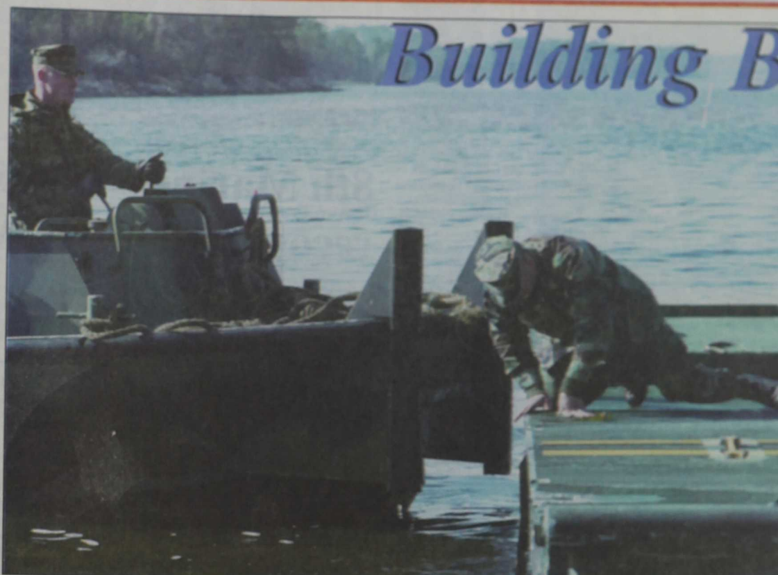
Lcpl Michael Dryden, left, and PFC Ernest Everman, both from Boat Co, 8th ESB, 2d FSSG, hook up an interior bay to a MK II Bridge Erection Boat before floating heavy equipment to MCAS New River.
