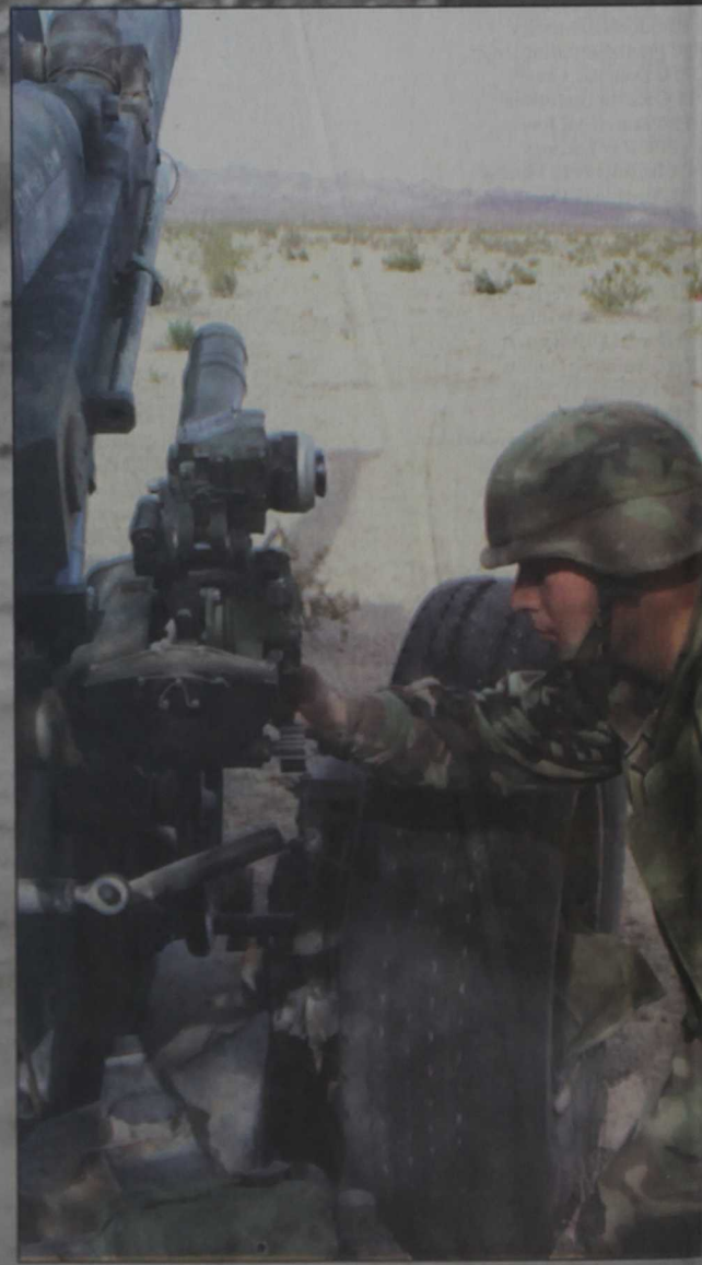
Warrenton, Mo., native Cpl Scott A. Gilliam, A-Gunner, Echo Battery, 2d Bn, sets the quadrant and deflection on an M-198 howitzer during a fire mission Jan. 23. The calibrations will ensure the rounds land on target.
