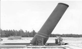
The largest caliber of artillery ever produced by the United States was the 914 mm mortar *Little David*. The mortar was not intended to be used as a combat weapon, instead it was used to test fire projectiles to study the ballistics of aerial bombs.
