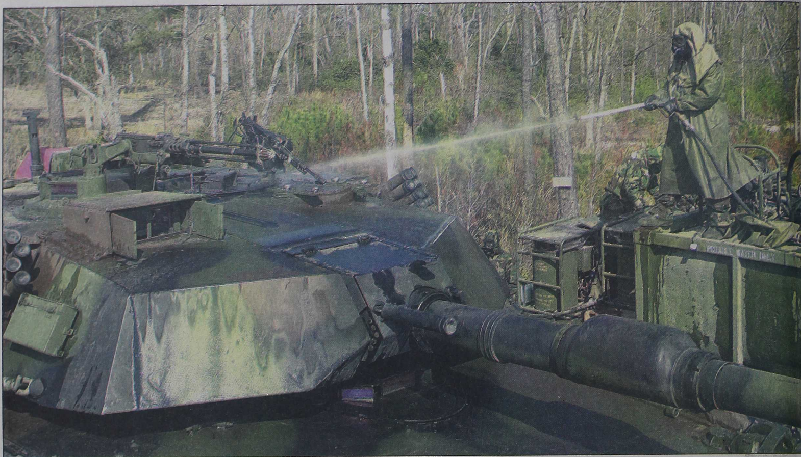
Using water for training purposes, Marines from 2d Tanks decontaminates their vehicles from high, low and all sides.
