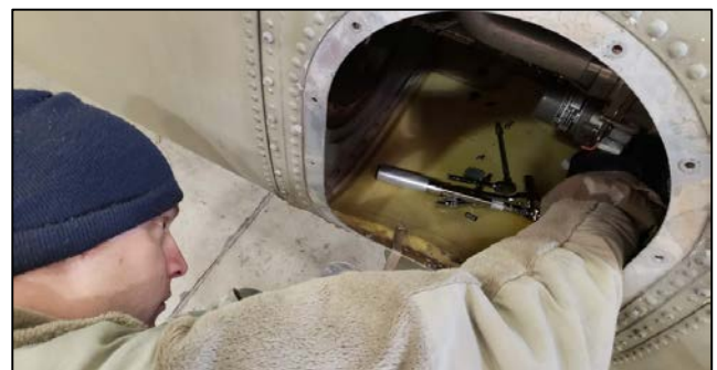
SPC Johnson of B Co. inspects the gaskets of a fuel tank for leaks during routine maintenance.
