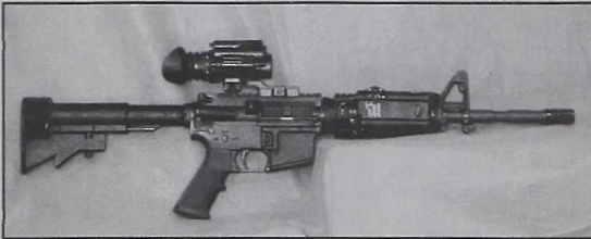
This M-4 is equipped with the rail adapter system, AN/PVS-14 sight and PAQ-4C
