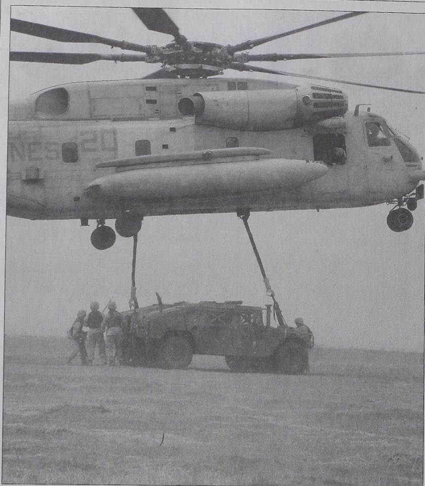
Marine Expeditionary Unit Service Support Group 15's Helicopter Support Team hooks up two "Hardback" High Mobility Multi purpose Wheeled Vehicles to a CH-53E 'Super Stallion' from Marine Heavy Helicopter Squadron 462. The exercise was performed at California Site 21 to showcase the CH-53E's capabilities for production personnel from the History Channel's Modern Marvels .
