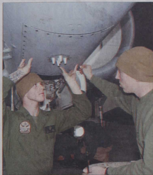
Al Asad, Iraq: Cpl. Skylar A. Colwell, an airframes mechanic with Marine Medium Helicopter Squadron 261 (Reinforced), holds up a panel on an AV-8B Harrier as Pfc. Kevin J. Lindsey, also an airframes mechanic with '261, screws it in. The Marines were finishing a routine inspection to ensure the aircraft was in flying condition.
