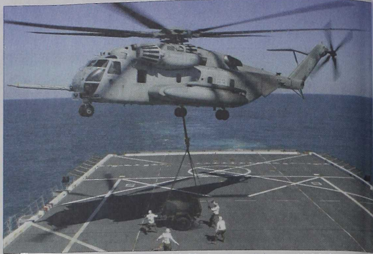
Combat cargo Marines from the 26th Marine Expeditionary Unit's Logistics Element, steady an external load for a CH-53E Super Stallion helicopter aboard USS San Antonio during the ship's Operational Evaluation. Photo by Cpl. Aaron J.
