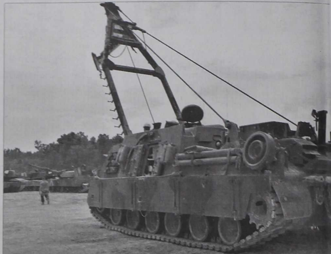
Tank mechanics depend on the M88A2 Heavy Equipment Recovery Utility Lift Evacuation System, or "Hercules," recovery vehicle. "Hercules pulls tanks out if they're stuck in ditches, or pulls them to safety if they're immobile due to an IED." Sgt. John L. Green, ramp chief for the company and a Denver, Colo., native.
