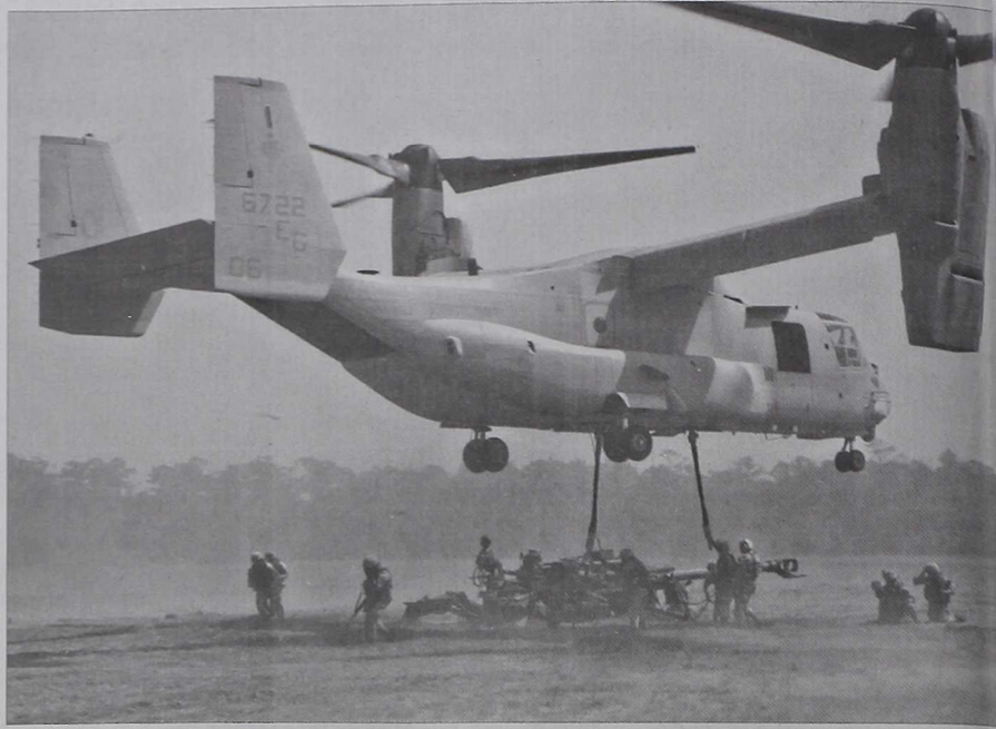
Marines with Battery S, 5th Battalion, 10th Marine Regiment, 2nd Marine Division, make Marine Corps demonstrating one of the tow capabilities of the MV-22 Osprey as it vertically lifts a 15,772 pound M19 Howitzer to another landing zone, Aug. 7. The demonstration was part of the battery's field exercise as they prepare for their scheduled deployment with the 26th Marine Expeditionary Unit. "It was the first time we've seen in the Marine Corps with the Osprey," said Gunnery Sgt. Nicholas Manganiello, the Battery Gunnery Sergeant. "We were able to do a pretty good lift with very minor damage. We can still put rounds down range, shoot, move and come back. That's our mission. As long as we can do that we are good." Lance Cpl. Ryan Turnage
