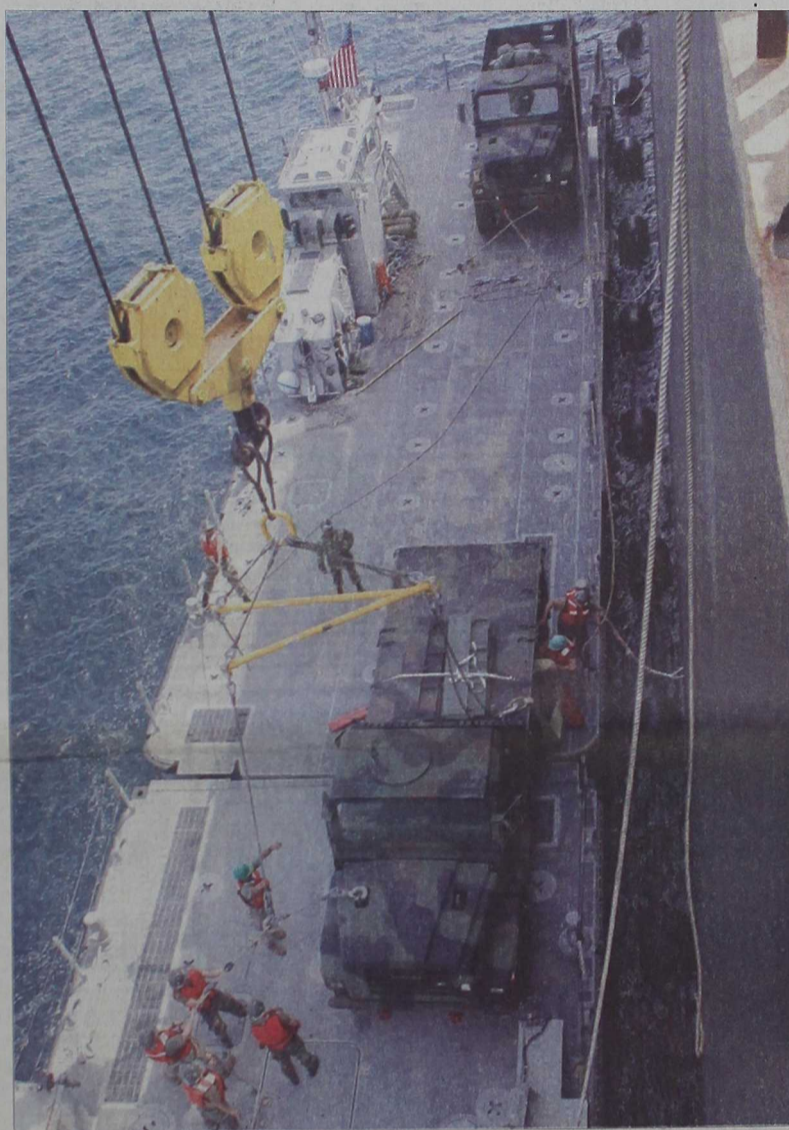
Marines from 4th Landing Support Battalion position a 7-ton Medium Tactical Vehicle as it is moved from the USNS 2nd Lt. John Bobo, a maritime prepositioning ship, onto the Improved Navy Lighterage System March 21. Rocco DeFilippis
