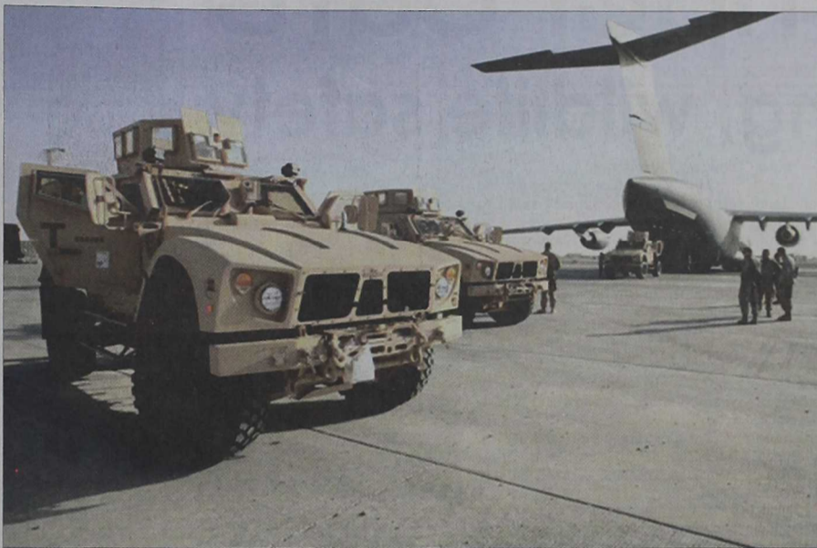
The newest addition to Marine Expeditionary Brigade-Afghanistan's motor pool, the Mine Resistant Ambush Protected - All Terrain Vehicle, arrived, recently at Camp Bastion in Helmand province, Afghanistan. The new vehicle provides crew members more survivability than its predecessor, the humvee.
