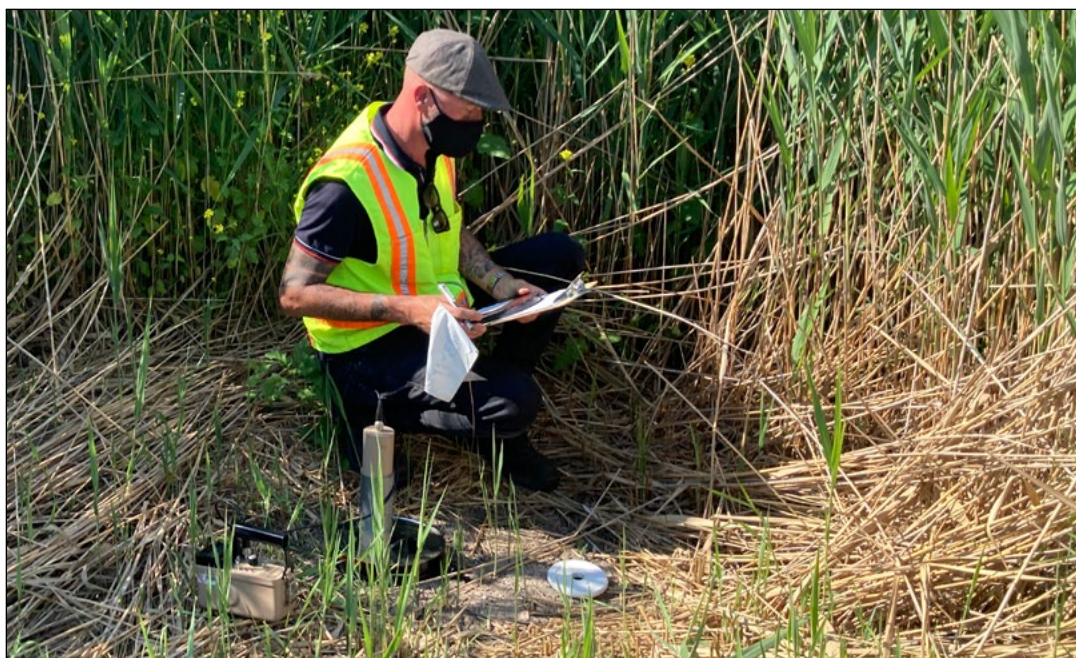
Shawn Andrews, health physicist, USACE Buffalo District, logs in the time of placement for a radon flux canister at the Tonawanda Landfill Vicinity Property.
