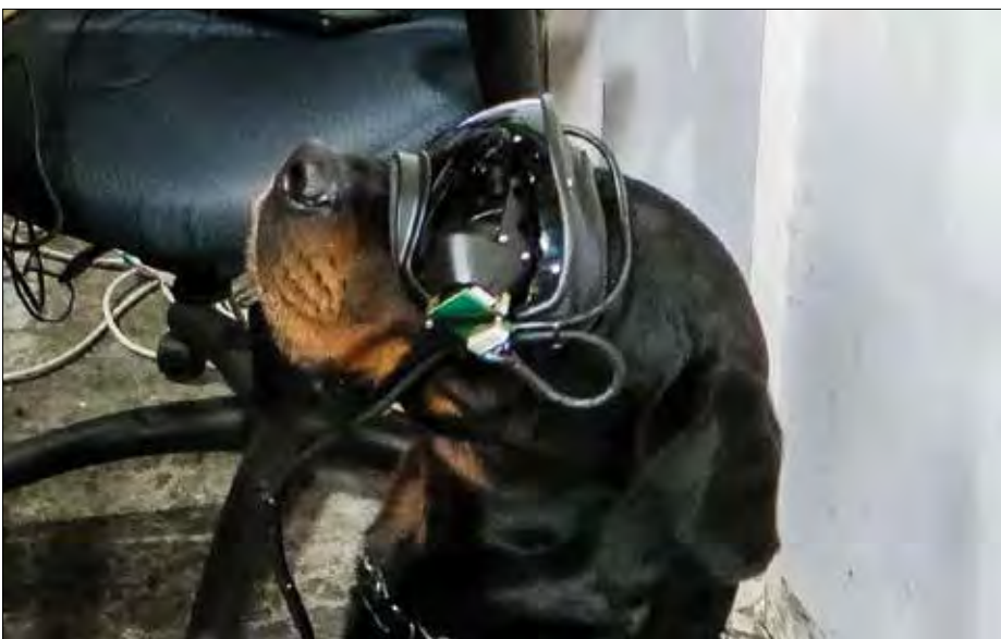
These augmented reality goggles are specially designed to fit each military working dog with a visual indicator that allows the dog to be directed to a specific spot and react to the visual cue in the goggles. The handler can see everything the dog sees to provide it commands through the glasses. (Courtesy Command Sight)
