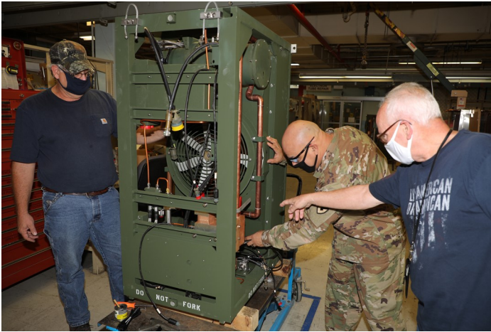
Chief Warrant Officer 3 Jesus Gonzalez (center) inspects solder joints on a cooling liquid electronic tube (CLET) in the reassembly process alongside Robert Hockenberry (right) and Brent Gordon (left) in the PATRIOT air-conditioner shop as part of the Training With Industry (TWI) internship at Letterkenny Army Depot. (U.S. Army photo by Pam Goodhart)
