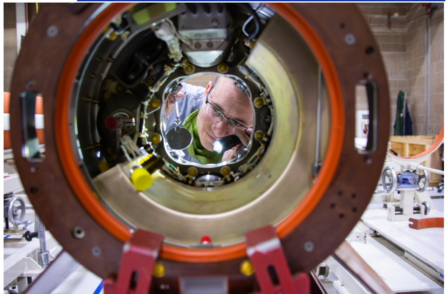
Justin Sites, an electronic technician in the Directorate of Missile and Aerospace readiness inspects the electrical components of a PATRIOT missile aft-body. (U.S. Army photo by Dorie E. Heyer, Public Affairs)
