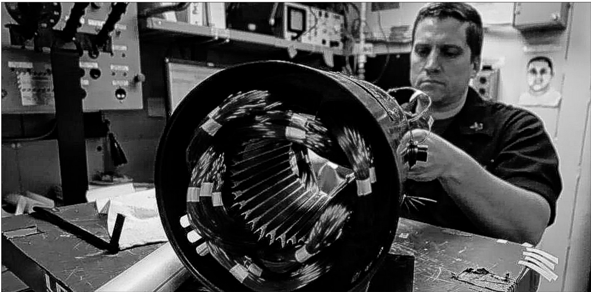
U.S. Navy photo Electrician Mates 1st Class Jacob Brown, from Dayton, Ohio, assigned to USS Gerald R. Ford's (CVN 78) engineering department electrical repair team performs assembly of a ventilation cooling fan motor prior to insulator varnish dip of the stator windings in Ford's Motor Rewind Shop May 13, 2020. Over 1,200 feet of wire is used to restore the 3 phase AC motor to rebuild the motor for certification testing/install.
