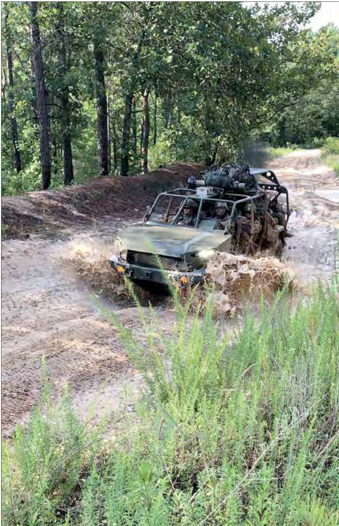
The ISV carries a nine-man squad, packs a payload of 3,200 lbs., can be externally sling loaded under Black Hawk and Chinook helicopters, is air droppable and provides exceptional mobility over all terrain. (Photo by Michael J Malik)
