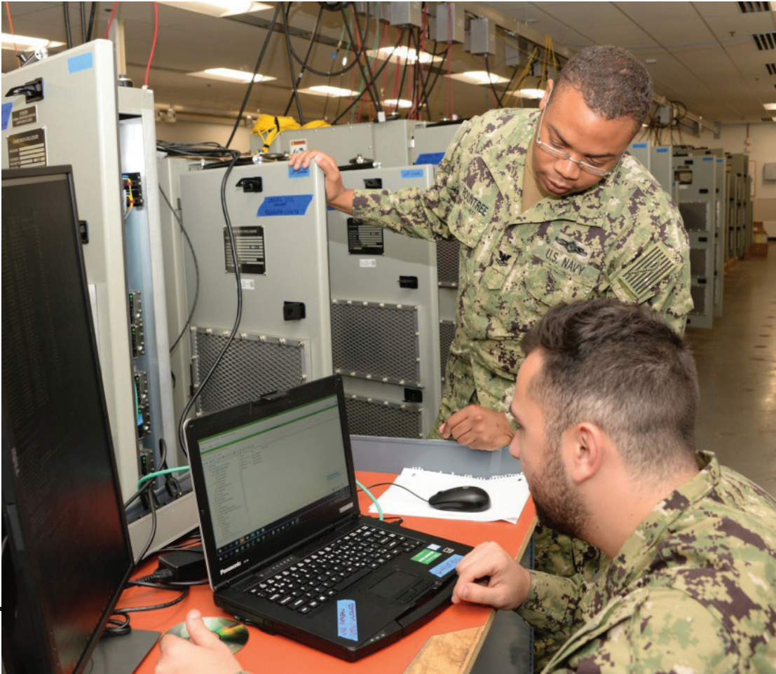
▶ U.S. Navy Information Systems Technicians 2nd Class Jchaun Rountree, standing, and Hakan Ozdemir, perform operational checks on Consolidated Afloat Ships Network Enterprise Services (CANES) racks bound for their ship, the aircraft carrier USS Ronald Reagan (CVN 76) in Naval Information Warfare Center Pacific's Network Integration and Engineering Facility. (Photo by Rick Naystatt)
