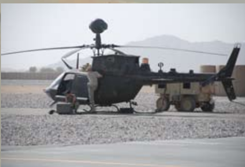
Task Force Saber Soldiers performing light maintenance on an OH-58D Kiowa Warrior Helicopter.
