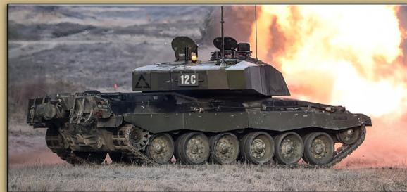
British main battle tank, first fielded in 1998. Four-man crew, 68.9 tons (82 tons with full add-on armor). L30A1 120mm rifled bore main gun, advanced Chobham armor protection. Upgrade options include modular hull and turret armor, an electronic countermeasures package and remotely controlled weapons system. In service with: United Kingdom, Oman.
