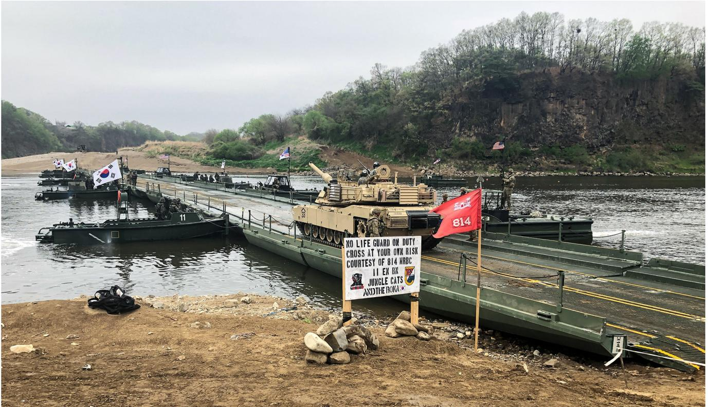
**Figure 2. An M1A2 tank from 3/1 ABCT crosses a hybrid IRB/SRB bridge constructed by members of 814<sup>th</sup> MRBC and 6<sup>th</sup> Engineer Brigade (RoKA) during a wet-gap crossing exercise. (U.S. Army photo by LTC Robert Dion)**
