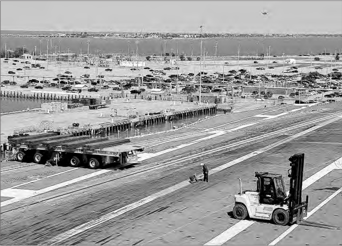
MC1 Jeff Troutman/ Personnel from Huntington Ingalls Industries-Newport News Shipbuilding Division measure and record inclination readings on USS Gerald R. Ford's (CVN 78) flight deck during a ship's weighted incline experiment at Naval Station Norfolk, April 16. The incline experiment helped calculate the ship's center of gravity, and will use information from the test to determine the ship's stability in a variety of design loading conditions.
