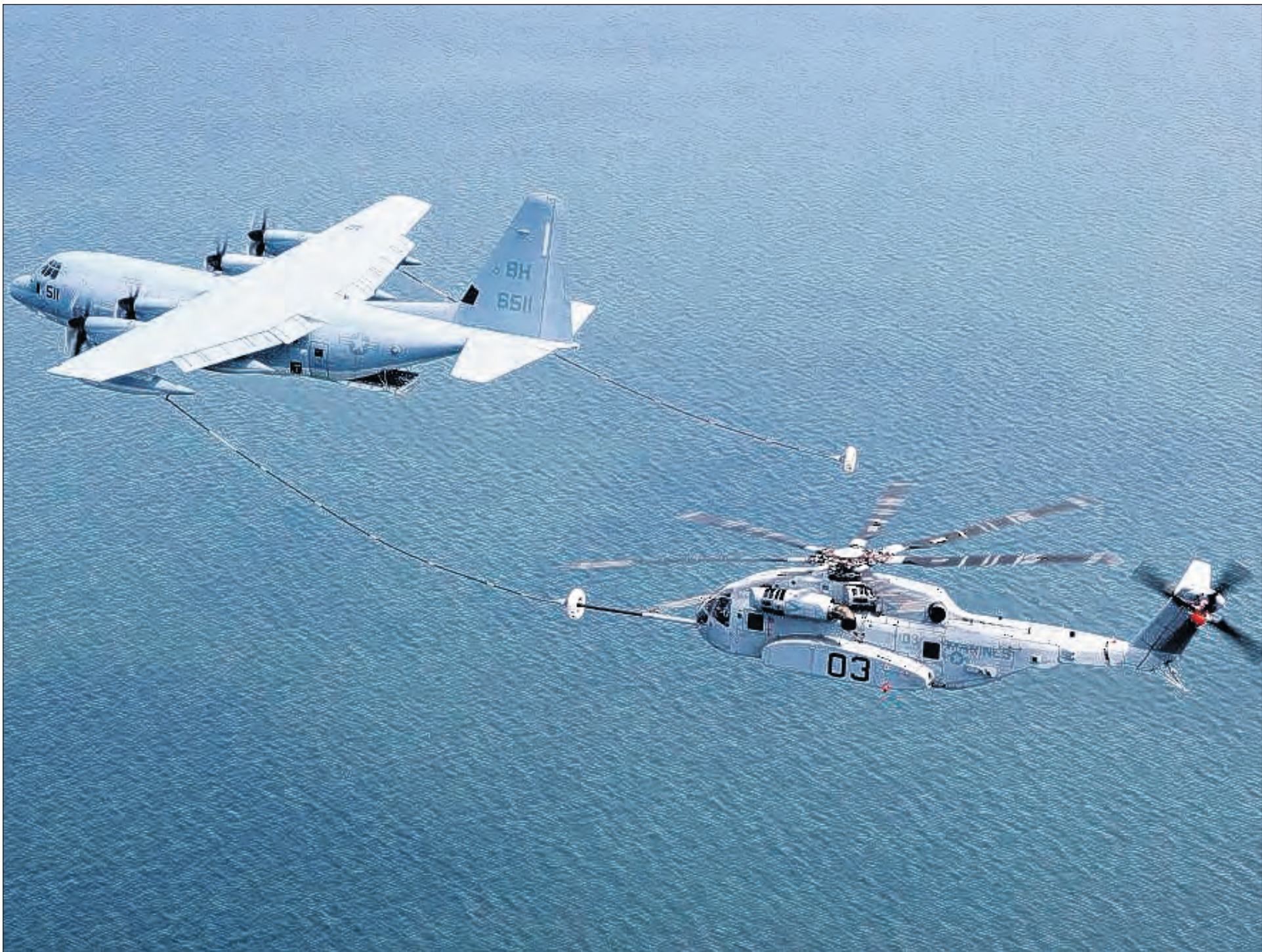
U.S. Marine Corps photo courtesy of Lockheed Martin A CH-53K King Stallion successfully plugs into a funnel-shaped drogue towed behind a KC-130J during aerial refueling wake testing, April 6, over the Chesapeake Bay. The all-new heavy-lift helicopter will expand the Marine Corps' ability to move more material more rapidly.
