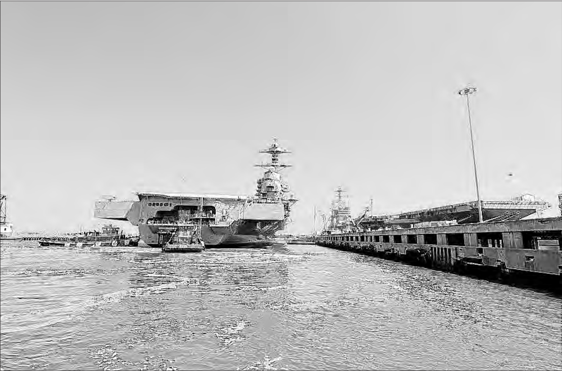
MC3 Brett Walker/ The aircraft carrier USS Gerald R. Ford (CVN 78), with personnel from Huntington Ingalls Industries-Newport News Shipbuilding Division, conducts a weighted inclining experiment at Naval Station Norfolk, April 16. The experiment helped calculate the ship's center of gravity, and will use information from the test to determine the ship's stability in a variety of design loading conditions.
