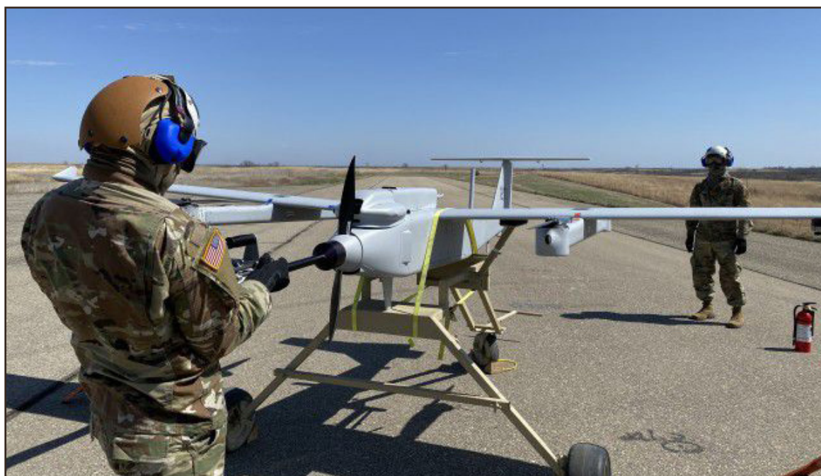
Spc. Christopher McCoy, assigned to 1st Engineer Battalion, 1st Infantry Division, conducts an engine start on the JUMP 20, as part of a Soldier touchpoint for the Future Tactical Unmanned Aerial System capability demonstration at Fort Riley, Kansas, April 8.
