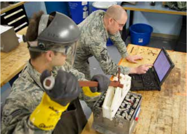
Left, Senior Airman Kenneth Purbeck, 446th Maintenance Squadron electrical and environmental technician, demonstrates how to operate the new battery cell extractor. Bottom left, the battery cell extractor in a maintenance workshop tool cabinet. Below right, Purbeck operates the battery cell extractor while Master Sgt. Robert Tingle, 446th MXS electrical and environmental technician, communicates the Air Force process on battery cell removal.
