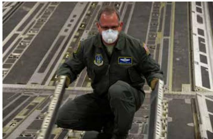
Senior Master Sgt. Robert Bertsch, a loadmaster assigned to the 446th Airlift Wing, Joint Base Lewis-McChord, Washington, flips cargo rails on the ramp of a C-17 to prepare the aircraft for a cargo upload during a local mission in late April. (Maj. Candice Allen)
