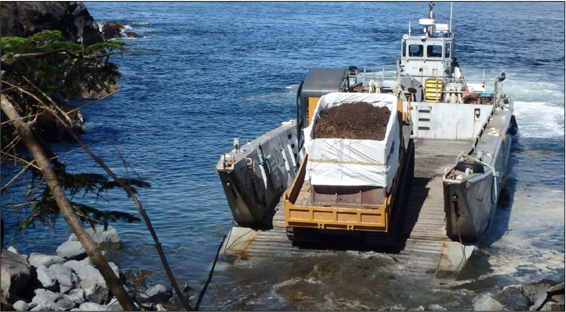
At the Fort Rouseau Formerly Used Defense Site a tracked dump truck, called a Marooka, is loaded with contaminated soil. In the back of the Marooka is a 5-cubic-yard bulk bag. The Marooka is being transported via a landing craft to another island. (Photo by A. Shewman)
