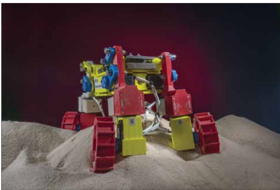
Built with multifunctional appendages able to spin wheels that can also be wiggled and lifted, a new robot developed at Georgia Tech with U.S. Army funding has complex locomotion techniques robust enough to allow it to climb sand covered hills to avoid getting stuck. (Photo by Christopher Moore, Georgia Tech)
