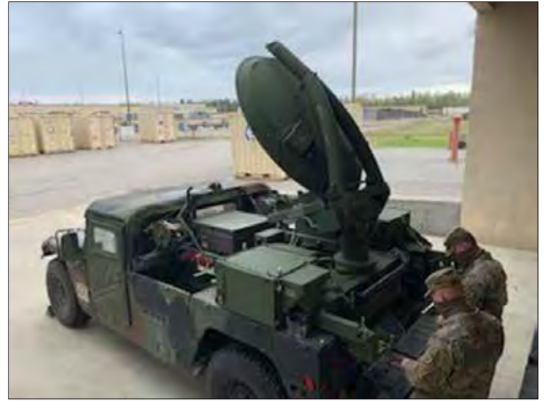
Spcs. DeLaRosa and Nunez raise the Secure Mobile Anti-Jam Reliable Tactical Terminal satellite. (Courtesy photo)
