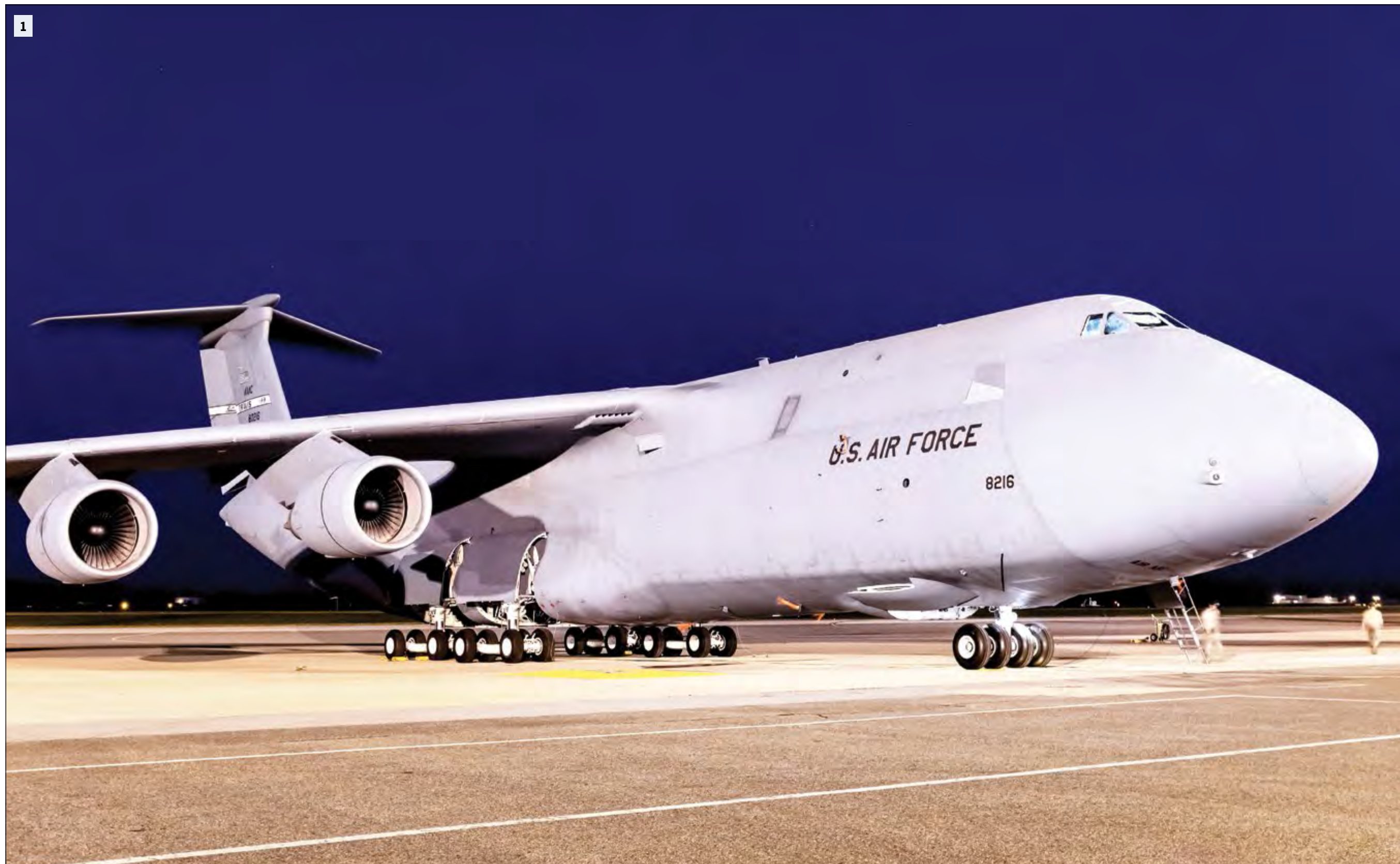
1) A C-5C Space Cargo Modified Galaxy from Travis Air Force Base, California, is parked on the flight line April 8 at Dover AFB, Delaware. The C-5C SCM has the troop compartment removed and a modification to the rear loading doors. It is specially modified to carry satellites and other large cargo.
